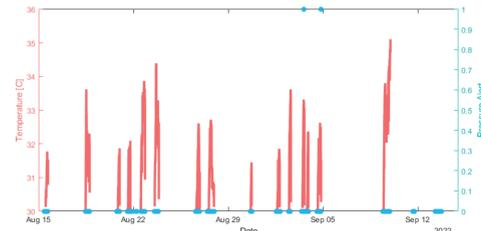
Figure 3. First metatarsal head temperature and pressure data collected from the sensory insole system. The patient was brought into the clinic presenting with an erythematous area suggestive of a pre-ulcer lesion on the plantar surface of the first metatarsal head.
