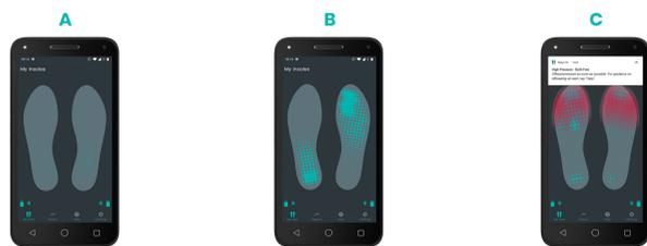
Figure 2. Proprietary Sensory Insole App – Frames A, B and C depict the main foot map screen of the app. These images illustrate an individual who has connected their insoles, who is walking or exerting pressure on their insoles, and who has received a high-pressure alert, respectively.
