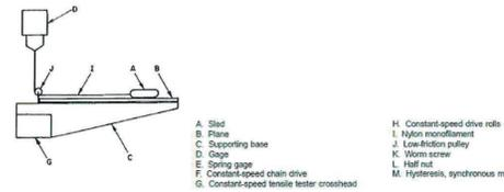
Figure 2 - Methods of assembly of Apparatus for the determination of Coefficient of Friction (ASTM D1894, Fig 1)
