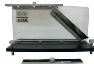
Figure 3: Shirley Stiffness Test Equipment
