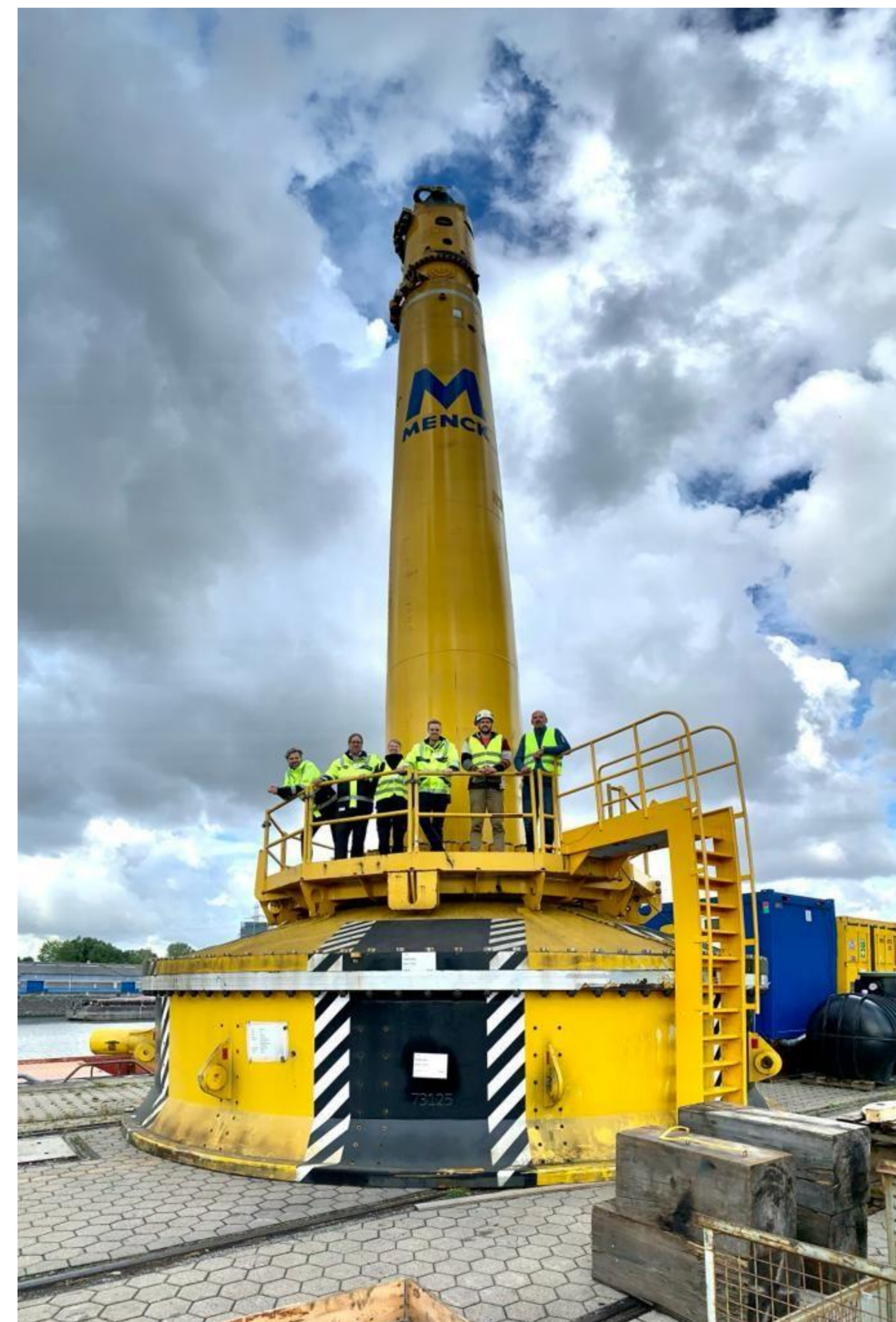
Menck 3500KJ hammer with Anvil for up to 7.5 meter diameter
