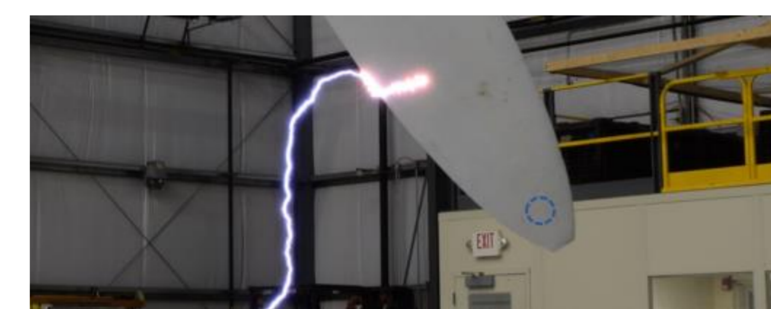
Bad result: puncture to down conductor
