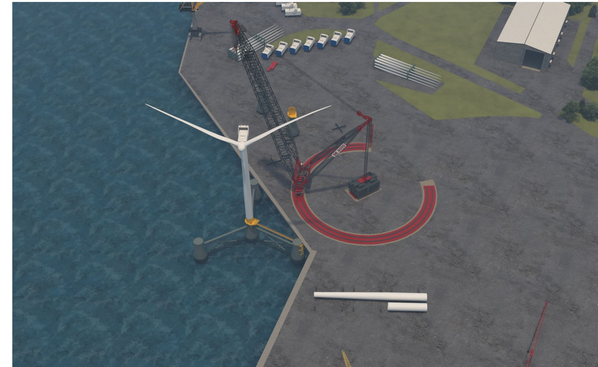
ABOVE: Mammoet's SK6,000 crane has the capacity to lift foundations directly from the quay to the water.
