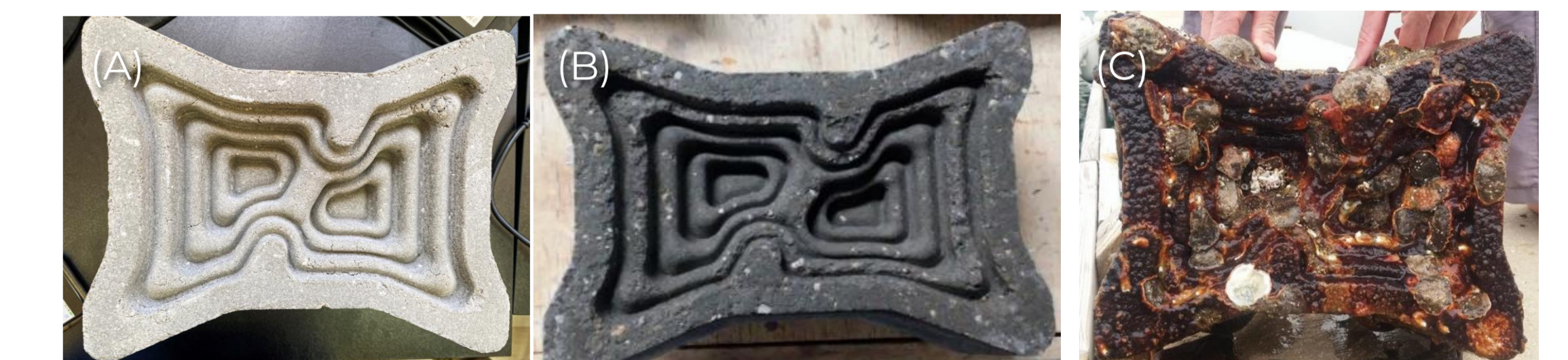
A sample of one ECO block. (A) New and untested, (B) after 75 freeze-thaw cycles, (C) after six months of submersion
