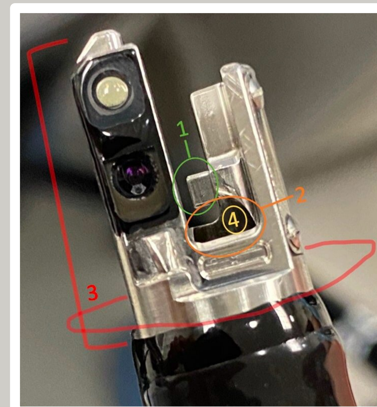
Figure 1. Sample locations: 1) The elevator tab 2) instrument channel distal opening 3) composite duodenoscope tip 4) the instrument channel
