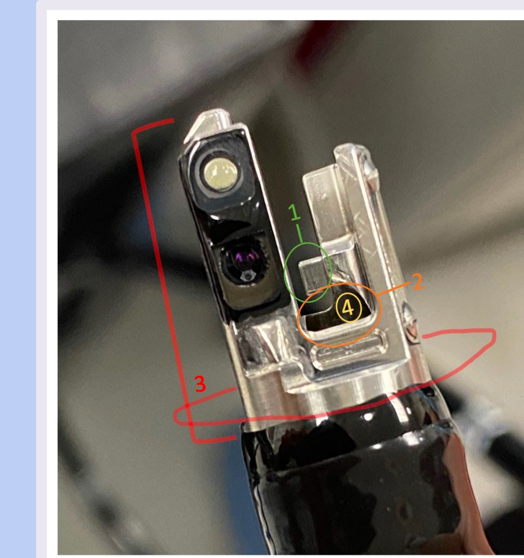
Figure 1. Sample locations: 1) The elevator tab 2) instrument channel distal opening 3) composite duodenoscope tip 4) the instrument channel
