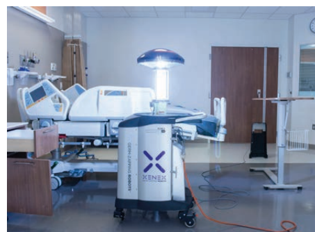
Figure 1: XENEX PX-UV robot completing disinfection in a hospital room (Photo: Business Wire)
