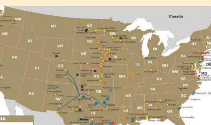
4,000 KM OF NH3 PIPELINE AND STORAGE TANKS are in place in Corn Belt, USA, for "green" ammonia fuel market rollout. NuStar Energy LP ammonia system (orange)
