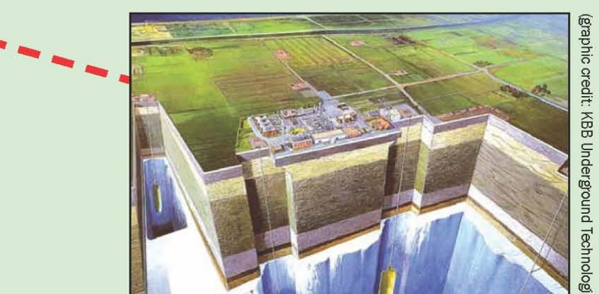
TYPICAL GH2 STORAGE CAVERNS IN DOMAL SALT: Multiple Caverns Share Surface Facility
