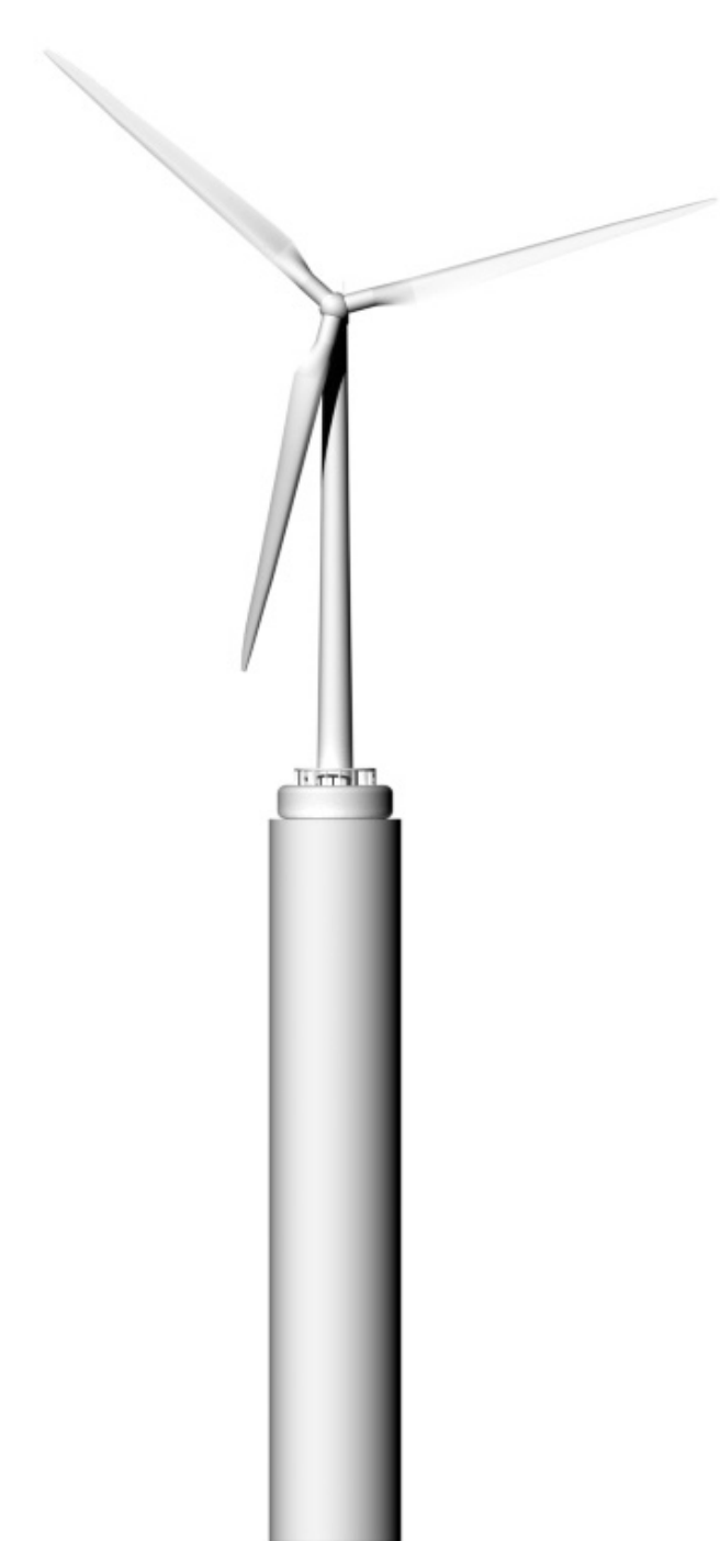
25 MW Turbine 300m x 26m Spar Installation
