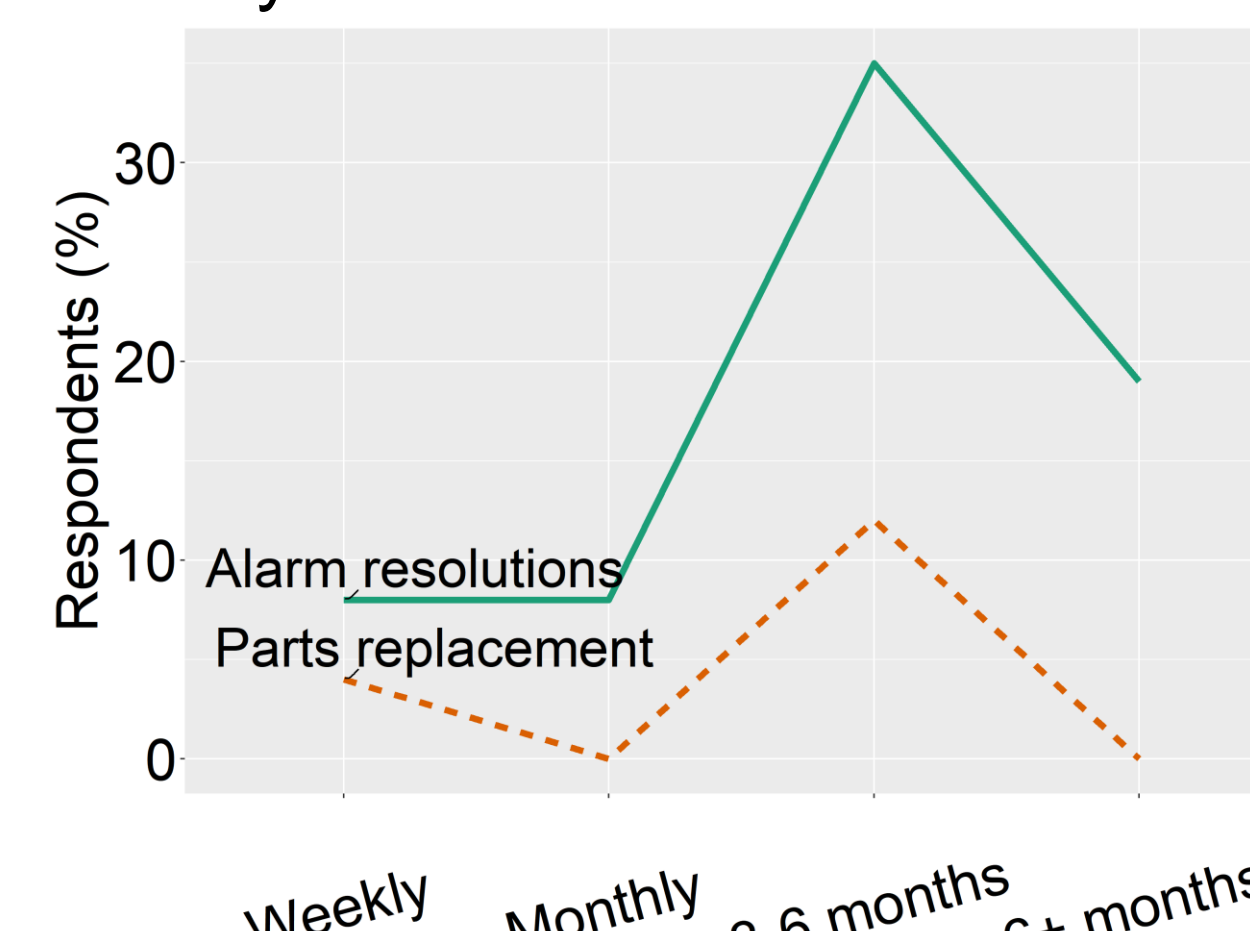
Figure 6. Frequency of corrective O&M. Alarm resolutions and parts replacement most often occur ~3-6 months.
