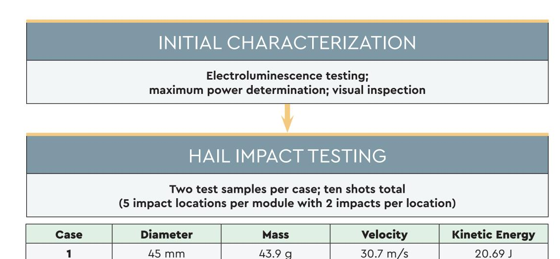
A side effect of thinner module glass is a decrease in hail-impact resistance. Glass manufacturers need a minimum thickness of roughly 3 millimeters to temper glass for maximum strength. The thinner 2mm glass used for many of today's large-format or bifacial modules is not conventionally tempered during manufacturing; it is heat-strengthened glass only, which increases the likelihood of breakage due to hail.
