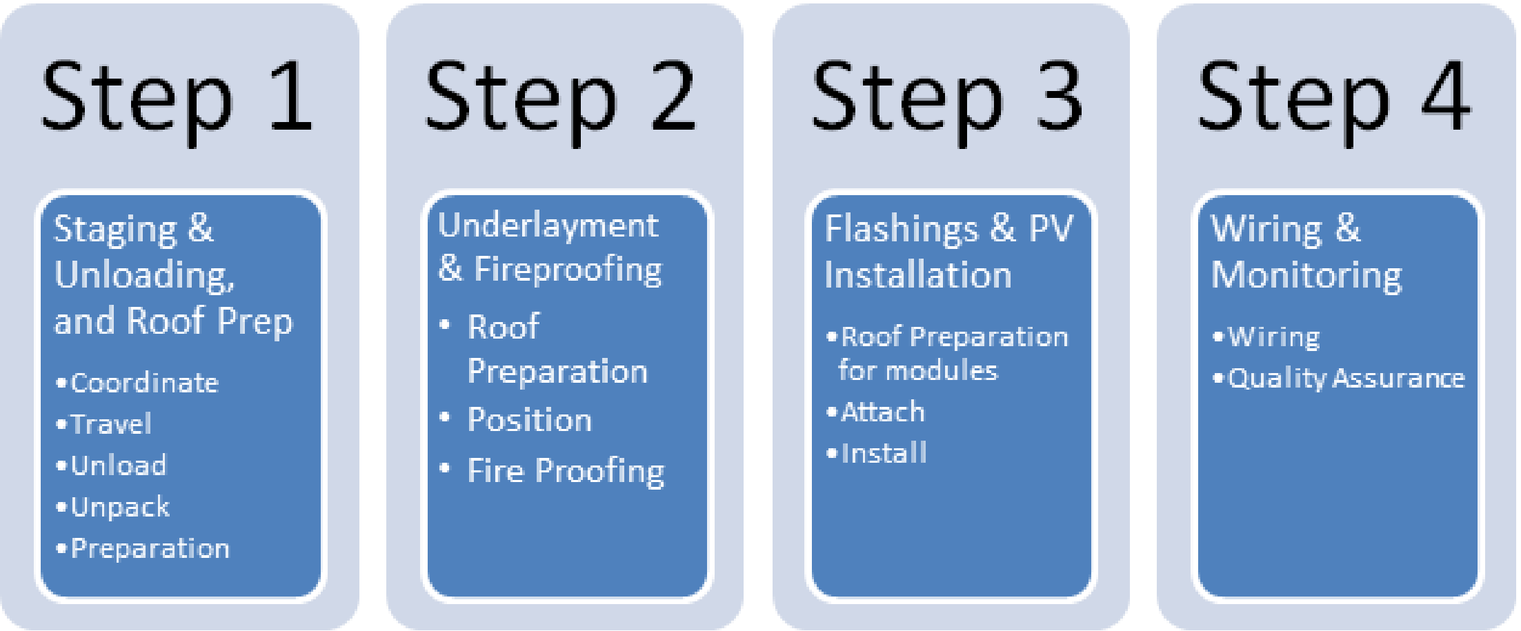
Figure 1. General BIPV Installation Process
