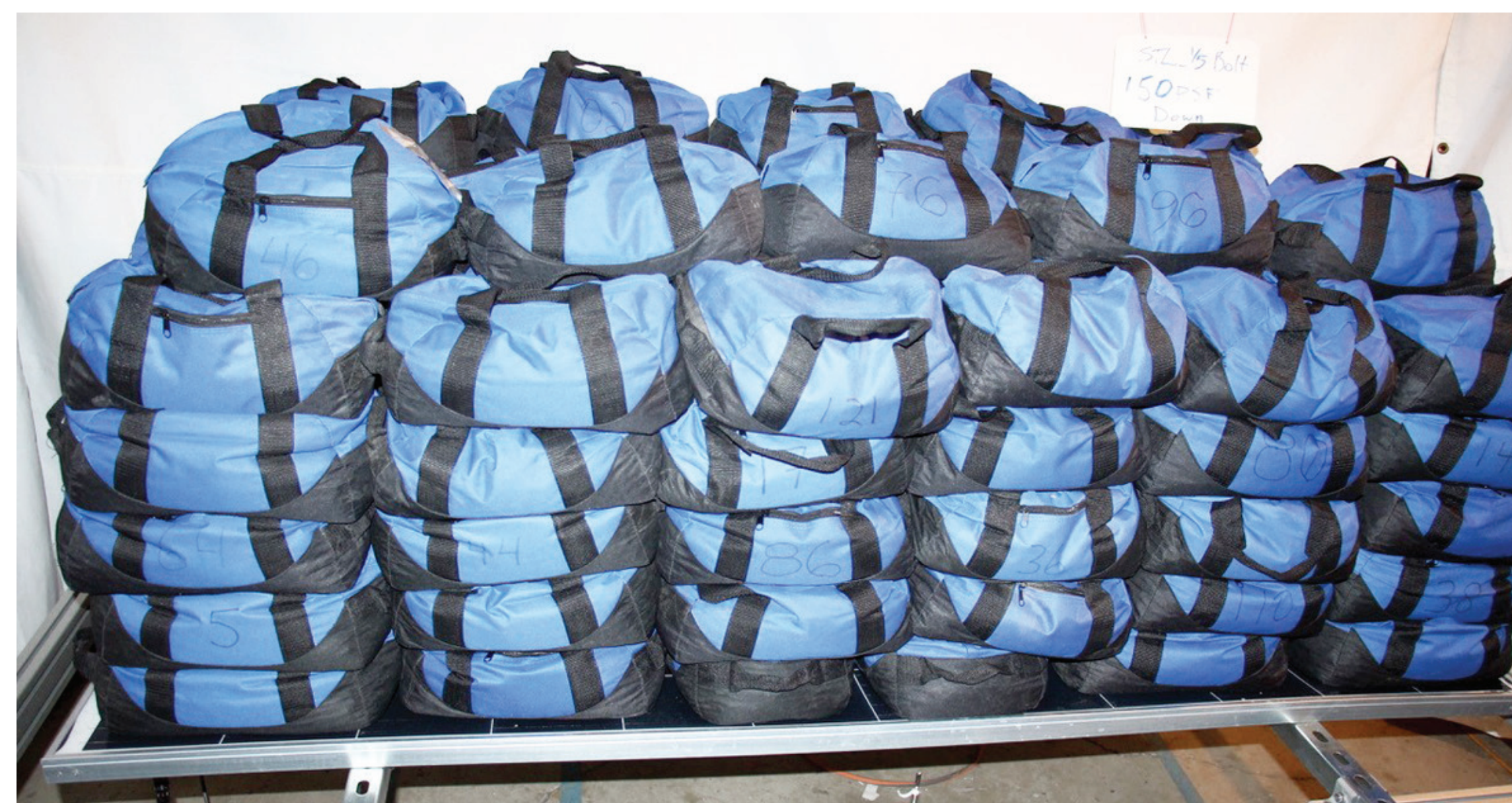
Image of Origami Solar's steel-framed module loaded with 150 psf (3200 lb)
