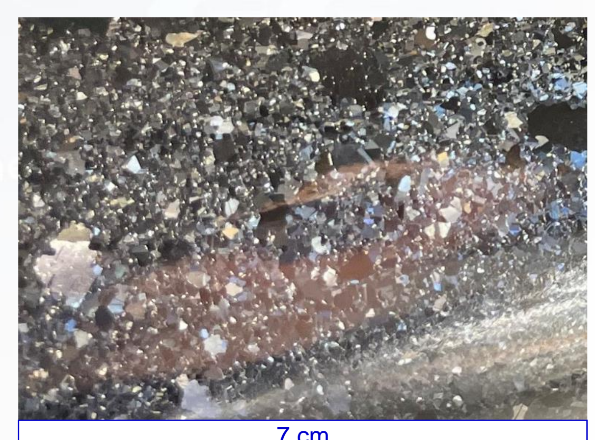
Optical image Contrast from individual Cu grains, graphene on top (not visible)
