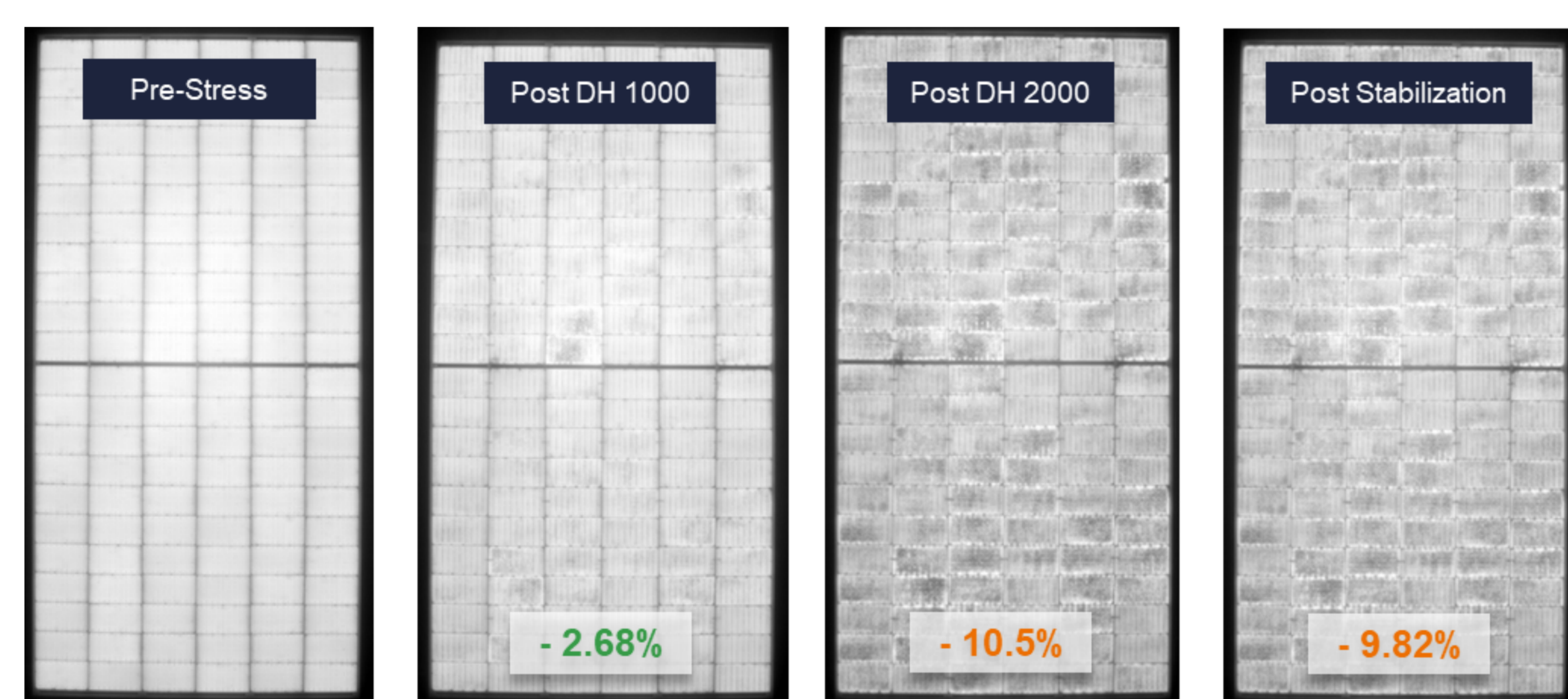
This gallium-doped BOM from 2021 was from the same manufacturer. No more BO destabilization, but a more traditional corrosion-based Damp Heat failure mode is apparent.
