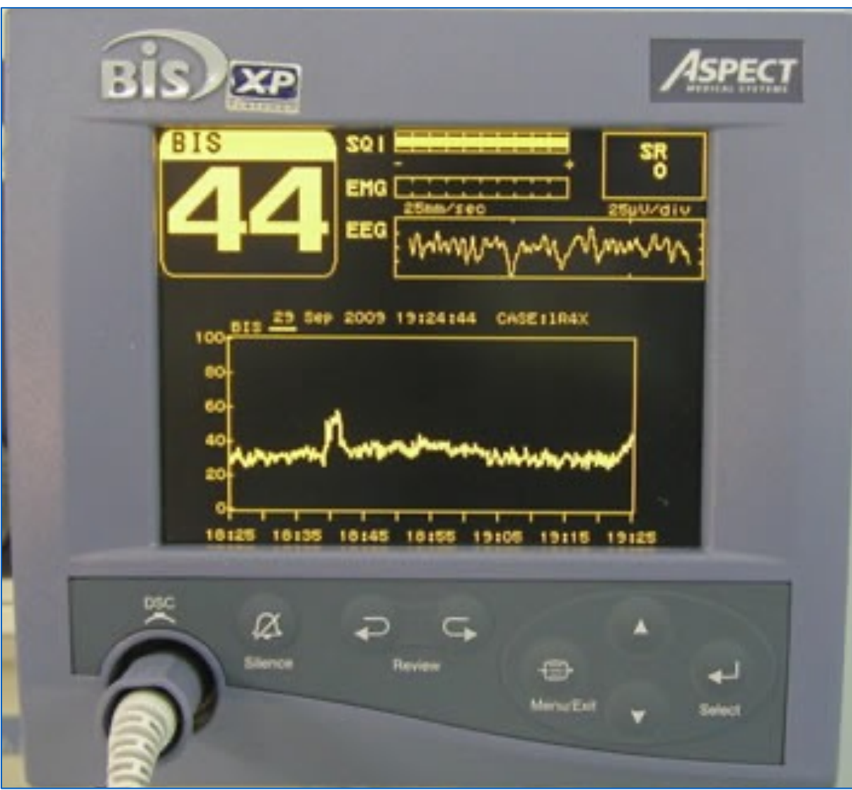
Figure 1: BIS monitor. The number on the top left corner of the BIS monitor depicts the BIS value. The BIS monitor will also measure both signal quality (SQI) and muscle activity (EMG) artifact as well as displaying the raw unprocessed EEG. The lower figure is the BIS trend over the last hour.
