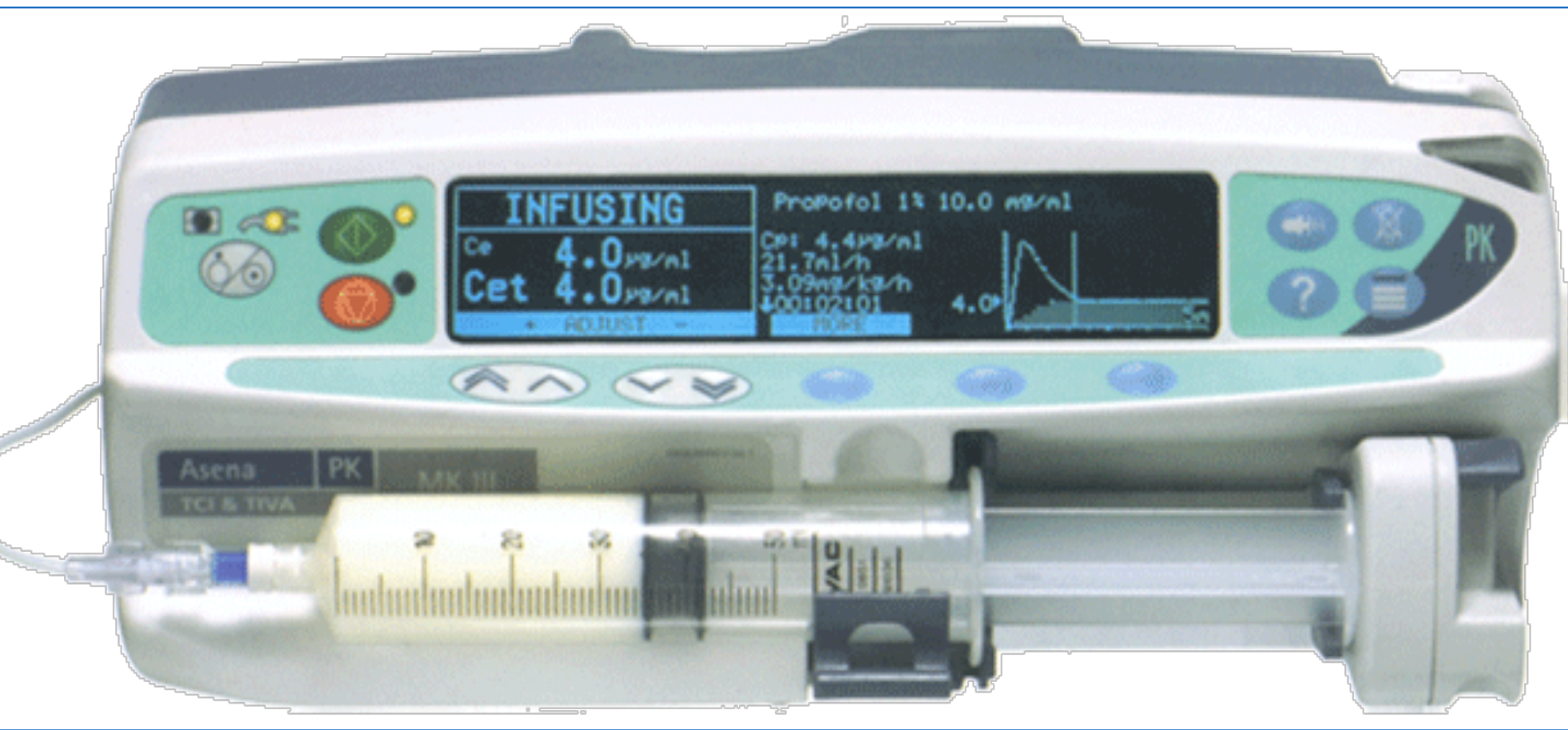
Figure 2: Propofol Infusion Pump. A medical device used to deliver measured quantities of medications to patients. The patient's weight, dose and drug concentration are entered and the infusion rate is calculated and displayed.
