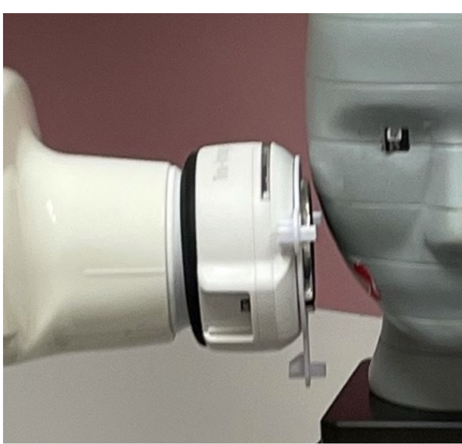
Figure 4. Tru-Image® Rectangular Collimator with the Pediatric Phantom
