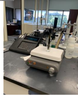
Figure 3. Measuring \text{Ca}^{++} with Orion meter with calcium electrode
